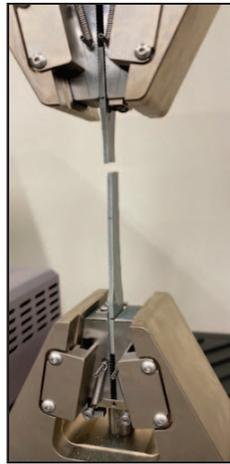
Figure 2: Short-term Flexural Testing
