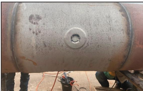
Figure 3: Hole-Spanning Testing Pipe Sample
