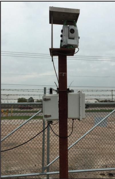
**Figure 5. Survey monitors were used for a detailed surface settlement monitoring program**
