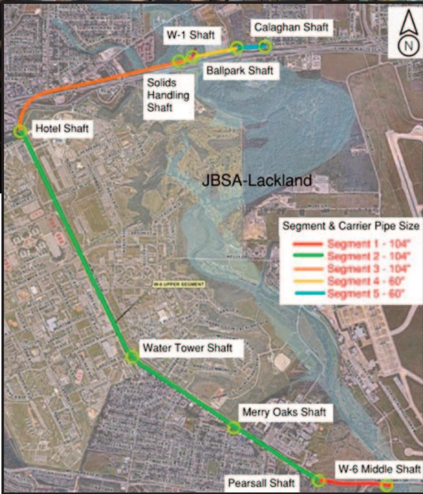
**Figure 1. SAWS W-6 Upper Segment Tunnel Alignment**
