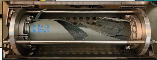
**Figure 6: Burst Pipe Sample**
