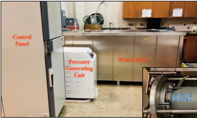
**Figure 5: Hydrostatic Pressure Testing Equipment**
