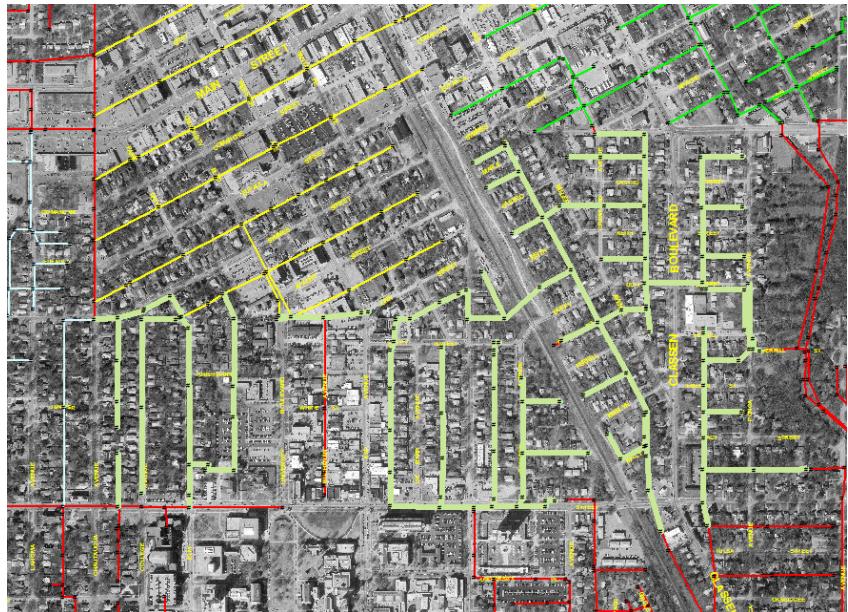
Figure 7: Year four still addresses oldest areas first draining into the Bishop Creek Basin, covering more than 30,000 linear feet
