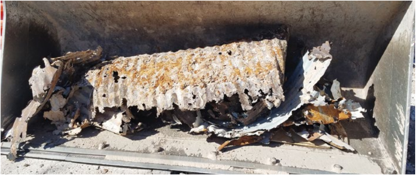
Figure 2 – Condition of the CMP
