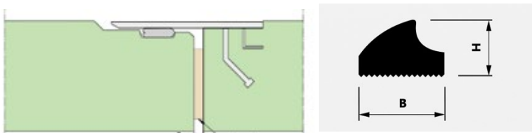
Figure 3 - Thompson Pipe Group Microtunneling Joint
