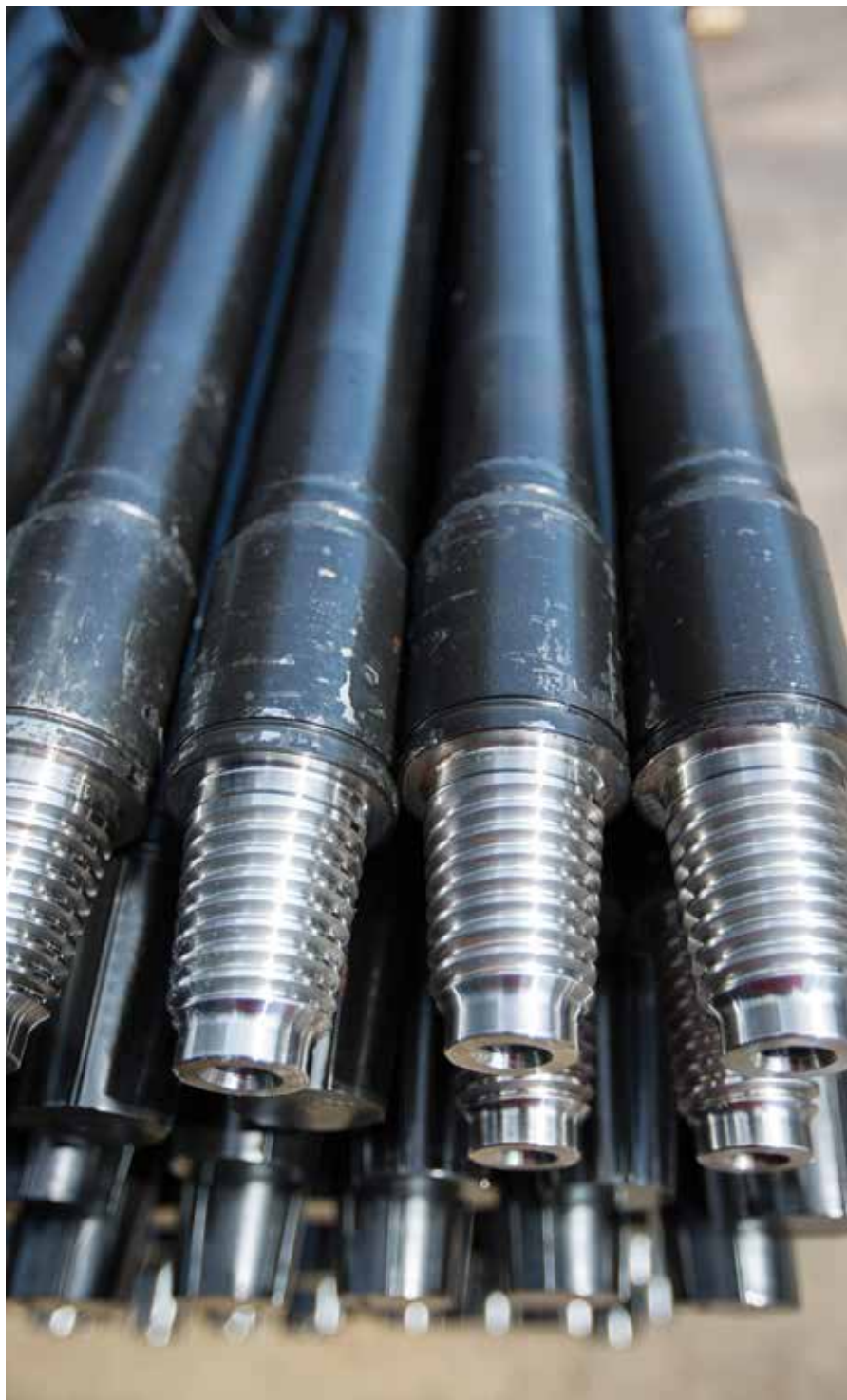
Consistent maintenance practices play a large role in getting the most out of drill pipe
